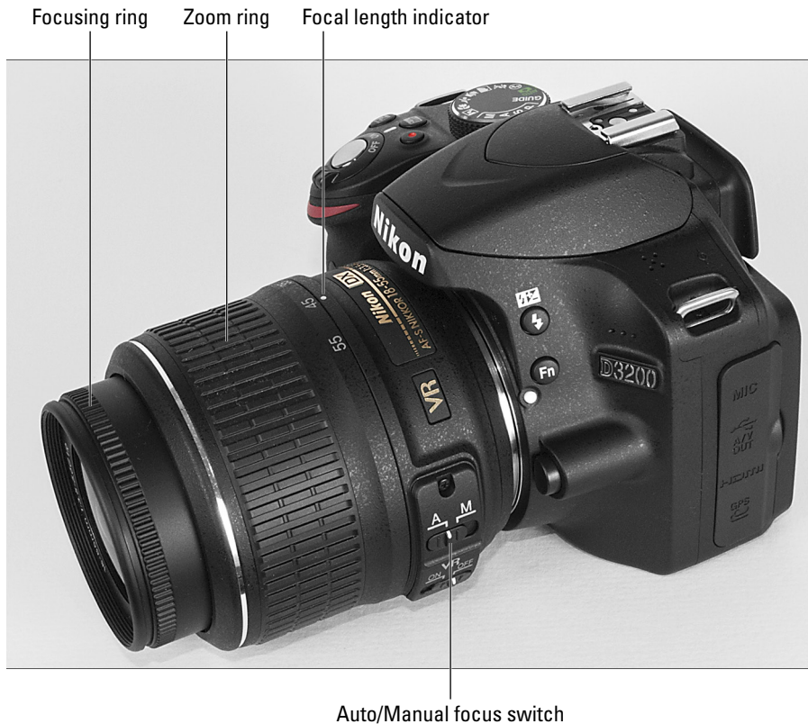
Figure 1-2: On the 18–55mm kit lens, the manual-focusing ring is set near the front of the lens, as shown here.
