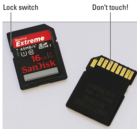
Figure 1-6: Avoid touching the gold contacts on the card.
