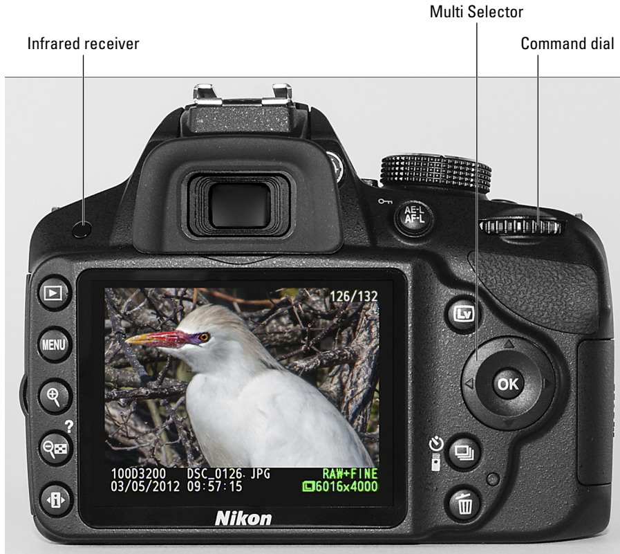
Figure 1-8: Use the Multi Selector to navigate menus and access certain other camera options.
