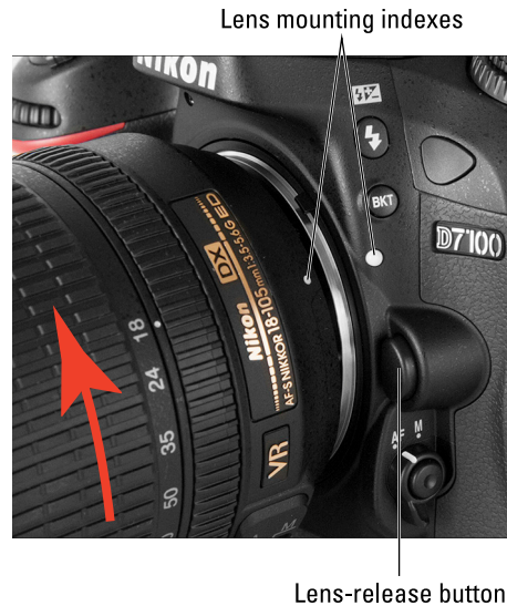
Figure 1-3: When attaching the lens, align the index dots as shown here.
