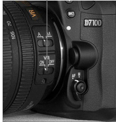
Figure 1-6: Turn on Vibration Reduction for sharper handheld shots, but turn off the feature when you use a tripod.
