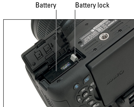
Figure 1-2: Push the battery down until it clicks in place.
